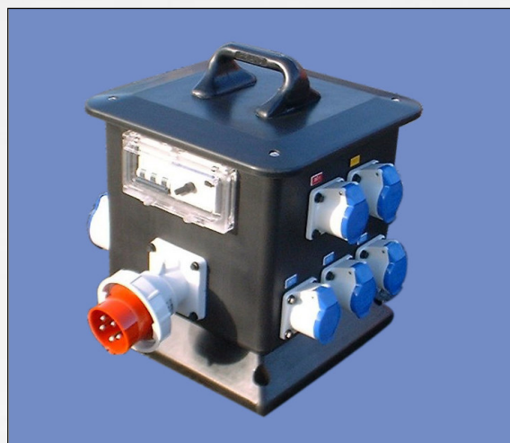
32A 5P 400V Appliance Inlet, 1 x RCD; Individual MCBs, 5 x 16A 230V Sockets, 3 x 32A 230V sockets
