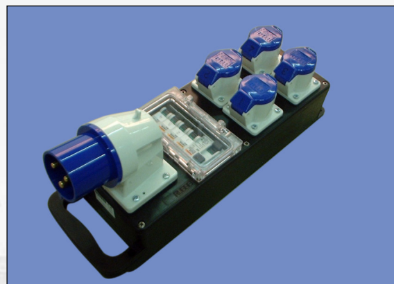
32A 3P 230V Appliance Inlet, 1 x RCD; Individual MCBs, 4 x 16A 3P 230V sockets
