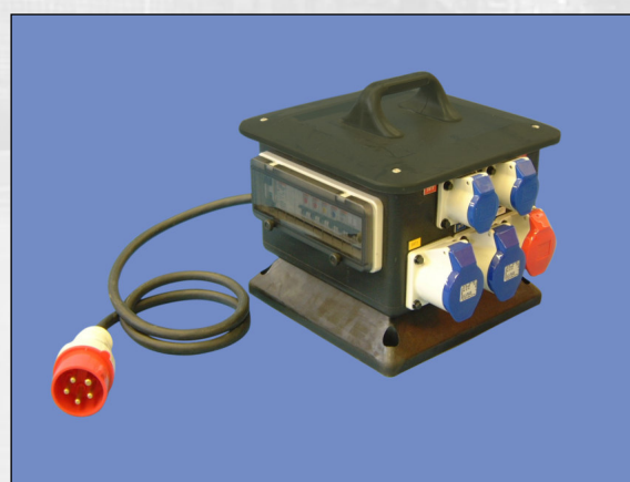
32A 5P 400V Plug + 1M 6mm 2 HO7 5C Cable, Multiple MCB / RCDs, 4 x 230V and 2 x 400V Sockets
