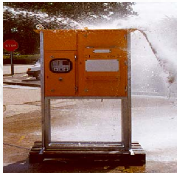
DSU UNDERGOING WATER INGRESS TEST TO COMPLY WITH IP56
