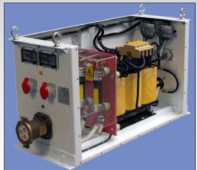
Combined assembly incorporating a 3300:400/110V 35 kVA transformer with 400V and 110V distribution (all covers removed)
