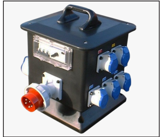
32A 5P 400V Appliance Inlet, 1 x RCD 5 x 16A and 3 x 32A 230V sockets / MCBs
