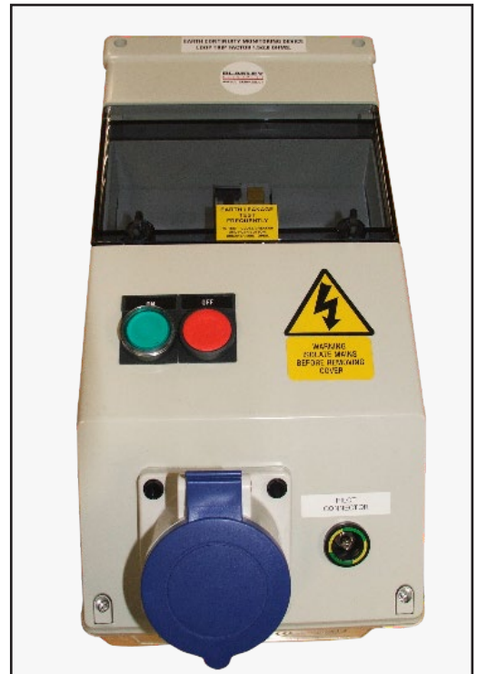
Assembly incorporating a 32A 230V mains socket, a POAG supplementary earth socket, RCD protection and monitored earth protection to BS4444.
