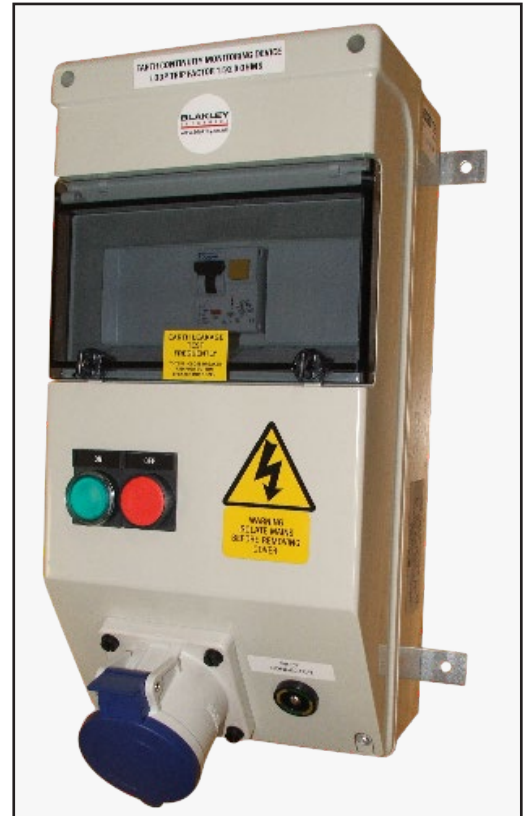
Assembly incorporating a 32A 230V mains socket, a POAG supplementary earth socket, RCD protection and monitored earth protection to BS4444.
