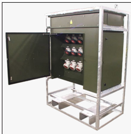
Free-standing, 800A rated, distribution assembly, mounted within a crash frame, fitted with 4 no. 125A sockets and 8 no. 63A sockets, individually protected by 4P MCB with variable time and current RCD protection
