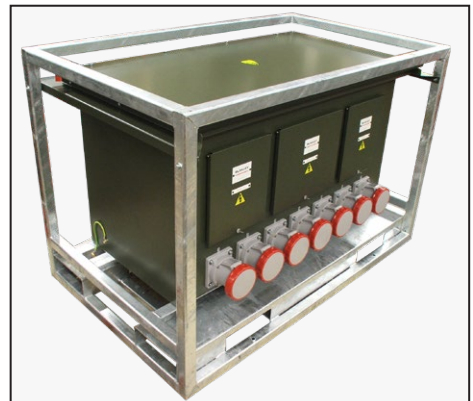
FEPS-LAPDS Generator Interface Unit enabling 3 no. 40kW FEPS generators to supply 7 no. 63A industrial socket outlets with RCD protection.
