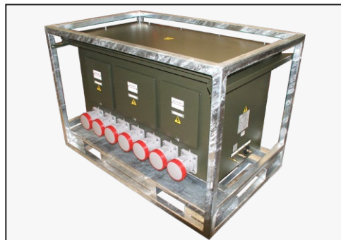
Generator Interface Unit supplied from military FEPS generators, fitted with protective crash frame and RCD protected industrial sockets
