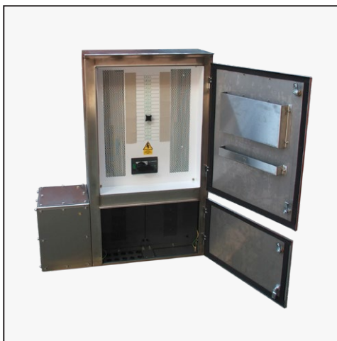
MCB board fabricated from 316L stainless. The internal inset panel incorporates mesh sections enabling MCB terminal temperatures to be accurately checked at any time with a thermographic camera
