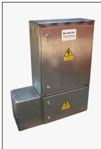
MCB board fabricated from 316L stainless. The internal inset panel incorporates mesh sections enabling MCB terminal temperatures to be accurately checked at any time with a thermographic camera
