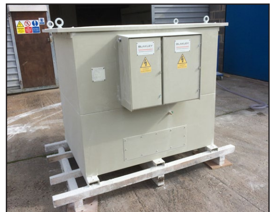
40 kVA IP55 Transformer after dust ingress type test
