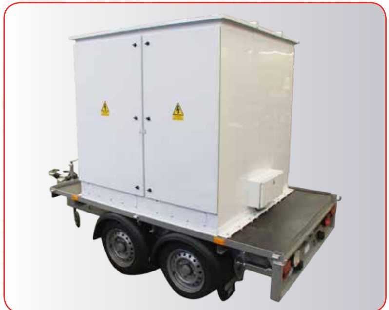
Distribution assembly mounted on road trailer
