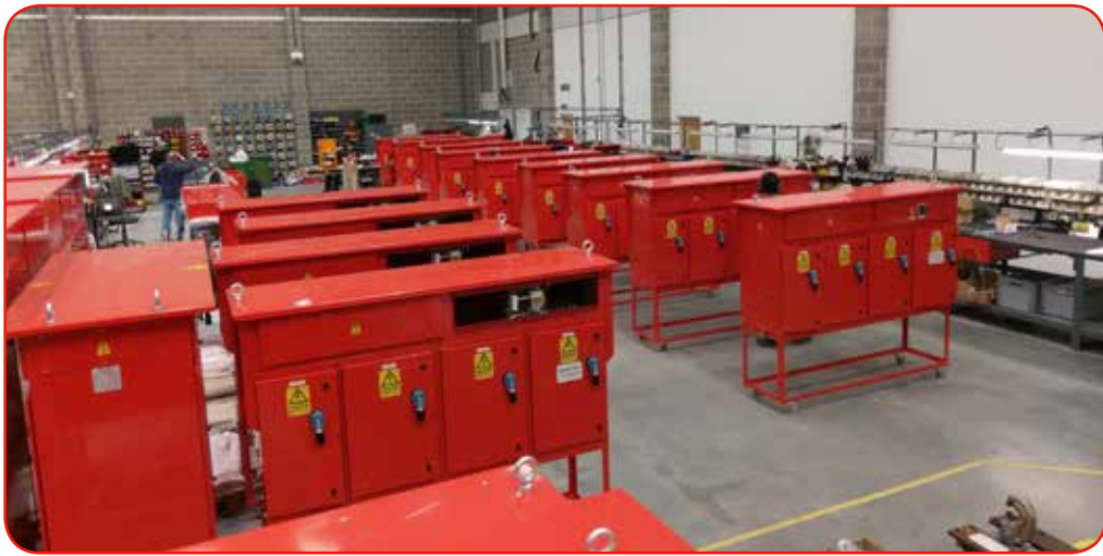
Final Assembly of 20 no. 400A Form 4 Type 3 Mains Distribution Assemblies nearing completion. Enclosures are fabricated from 316L stainless steel with a conspicuous painted finish, shade Poppy Red to BS4800 04 E 53.
