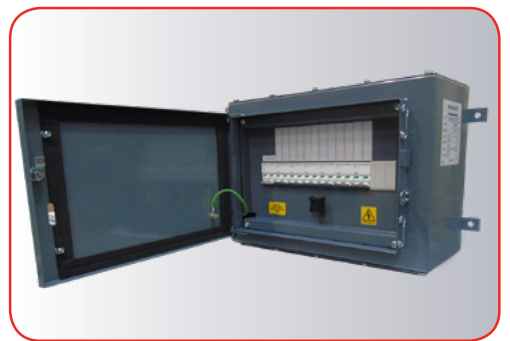
Part S040392, MCB Board, 110V, fitted with a 100A incoming isolator and 6 no. 16A DP Type "C" MCBs
