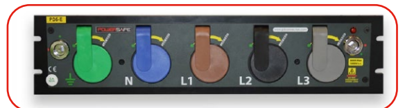
Optional sequential powerlocks where connectors must be connected / disconnected in sequence (earth is first in and last out)
