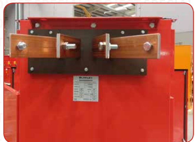
Connections for testing bus bar system
