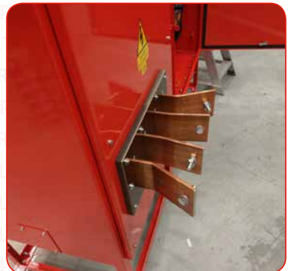
Special Incoming Termination Arrangement
