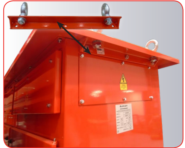
Lifting Arrangement as fitted to B6 / B7 series MDAs, with a Safe Working Load of 750kg per pair. Eye bolts are the fixed type and certified to BS4278
