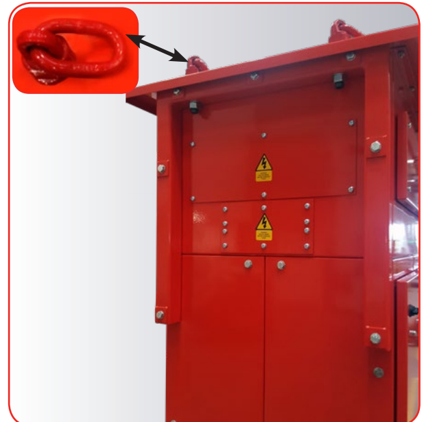
Lifting Arrangement as fitted to a B8 series Mains Distribution Assembly, with a Working Load limit of 2000kg per set of 4. Eye bolts are swivel type and certified to BS 4278.
