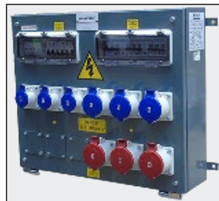
Part No. S171041, 100A 4P Switch, 3 x 32A 400V, 3 x 32A 230V & 3 x 16A IP44 Sockets with RCBOs
