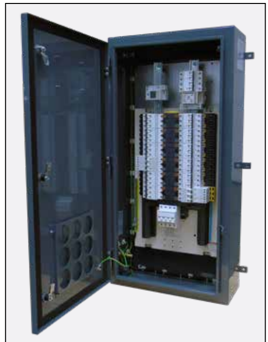
IP66 Distribution Board, 125A, 12W, TP&N c/w DIN rail
