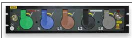
Optional sequential SP connectors which must be connected / disconnected in sequence (earth is first in and last out)
