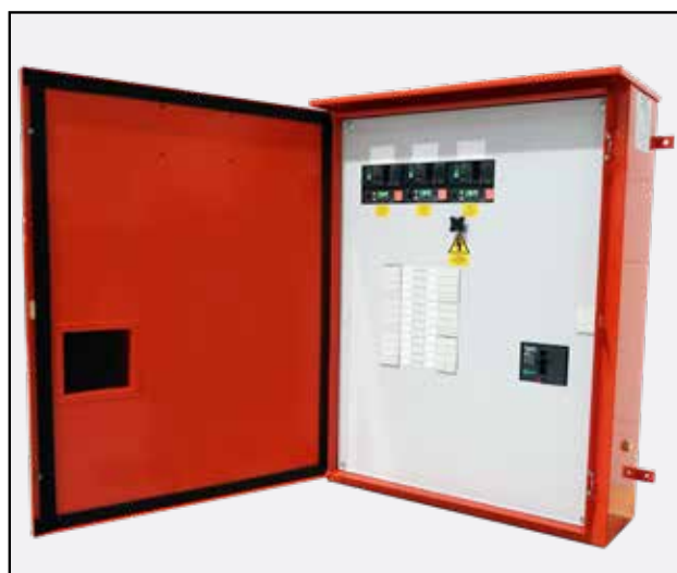
S140490R 200A MDA fitted with 3 no. 160A CBRs and an 8 way TP MCB pan assembly
