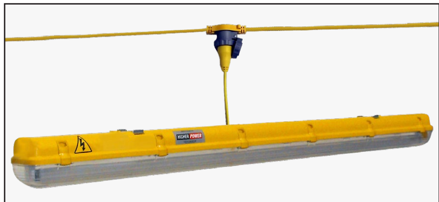
Flori-67 Plug-in, LED, 110V Lighting System. Versions available with 3 pin and 4 pin connectors (the 4 pin version enabling emergency fittings to be switched off without the risk of discharging or damaging batteries).
