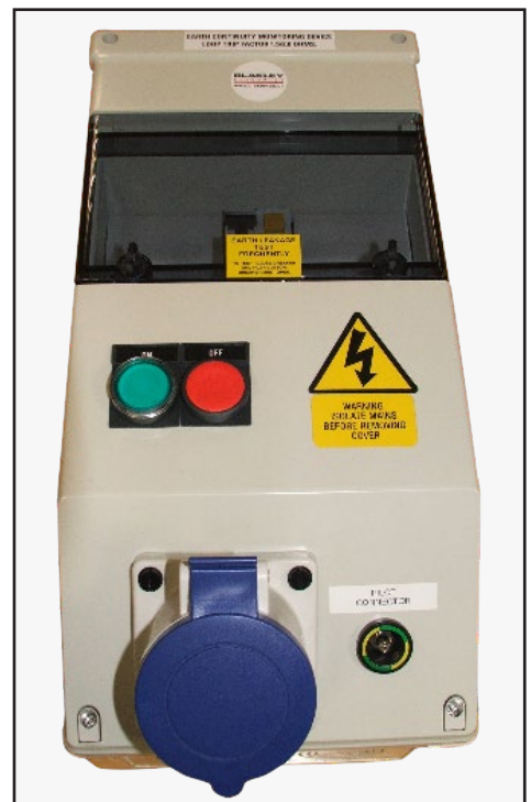
Part S190408 incorporating a 16A 2P+E 230V mains socket, a POAG supplementary earth socket, DP 30mA RCCB to BS EN 61008, SP MCB to BS EN 60898 and monitored earth protection to BS4444.
