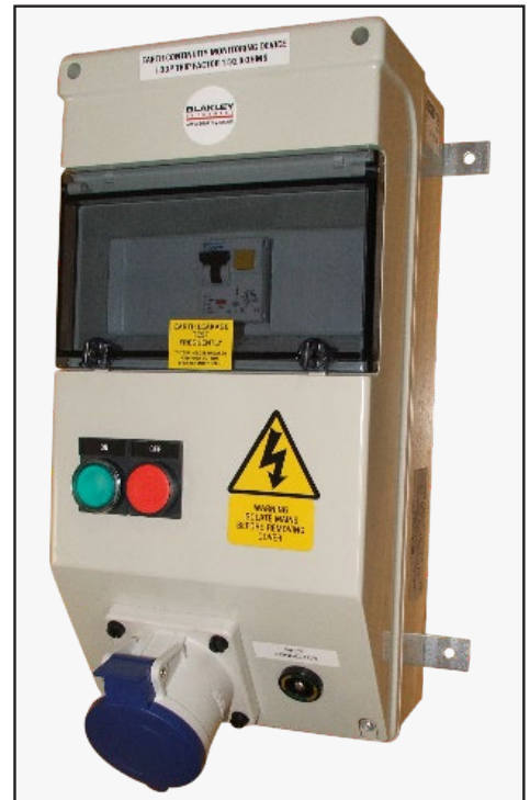
Part S190408 incorporating a 16A 2P+E 230V mains socket, a POAG supplementary earth socket, DP 30mA RCCB to BS EN 61008, SP MCB to BS EN 60898 and monitored earth protection to BS4444.
