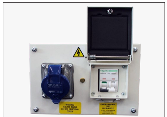
S120314 - LV Maintenance Socket, 16A, 230V, with integral 16A 30mA RCBO with shield plate removed
