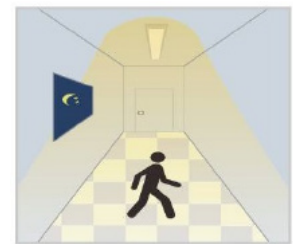
2. With light level detection off or when light levels are low, movement in the vicinity causes the light to turn on.
