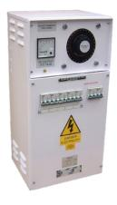
Variable Laboratory Supply Units (VLSUs) provide a separated extra low voltage supply, which enable experiments to be carried out in safety. They provide an AC or DC output, which is selected from a switch at the front of the assembly. The output voltage can be adjusted from 0 to 20V via a Variac and analogue voltmeters and ammeters display the voltage and current at the VLSU output terminals.
