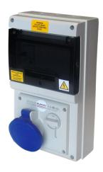
A range of all-insulated, IP44 rated, RCD protected socket outlets to BS EN 60309-2, with or without mechanical interlock, in current ratings of 16A and 32A and voltages of 110V, 230V and 400V.
