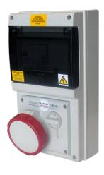
A range of all-insulated, IP66 rated, RCD protected socket outlets to BS EN 60309-2, with or without mechanical interlock, in current ratings of 16A, 32A, 63A and 125A and voltages of 110V, 230V and 400V.
