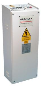
Safe Supply Unit in floor standing console style enclosure, 3 or 5 kVA rating, 1.25mA or 5mA sensitivity, 3 no. outgoing DP MCBs.
