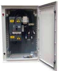
Earth leakage protection assemblies with overcurrent protection, rated from 100A to 1600A, 4P, housed in IP55, all insulated enclosures. All models incorporate variable sensitivity and variable time delay.
