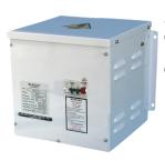
Safe Supply Unit in wall mounting enclosure, 2 or 3 kVA rating, 1.25mA or 5mA sensitivity, option of 2 or 3 outgoing DP MCB ways.
