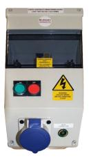
Monitored earth / RCD protected socket assemblies with integral POAG sockets, for 230V single phase or 400V three-phase applications, in current ratings of 16A, 32A, 63A or 125A.
