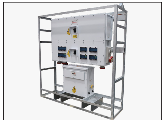
63A 400V sockets are switched and interlocked. Hard wired 110V circuits for tunnel lighting and sockets for power tools
