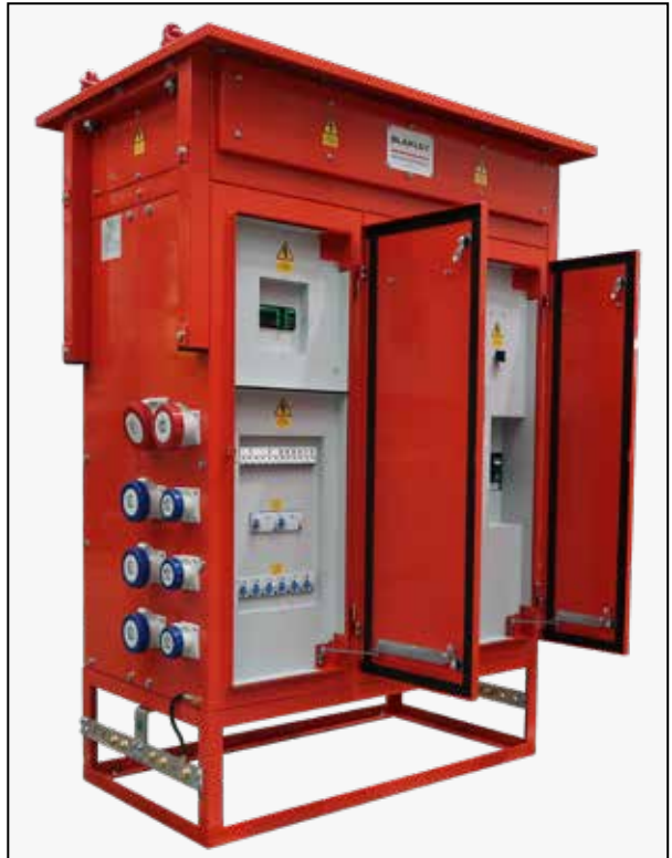
Part Number A7194411 630A MDA with MCCBs and bus bars segregated to Form 4A Type 3
