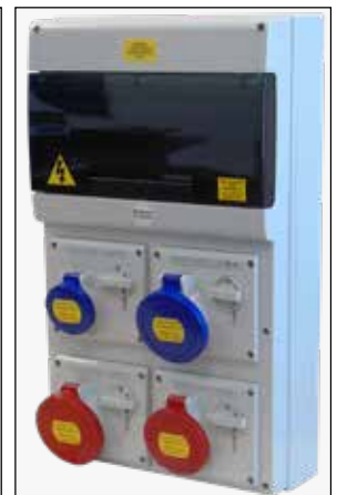
100A incoming switch fitted with 1 x 63A, 32A and 16A 400V socket and 1 x 32A and 16A 230V socket.
