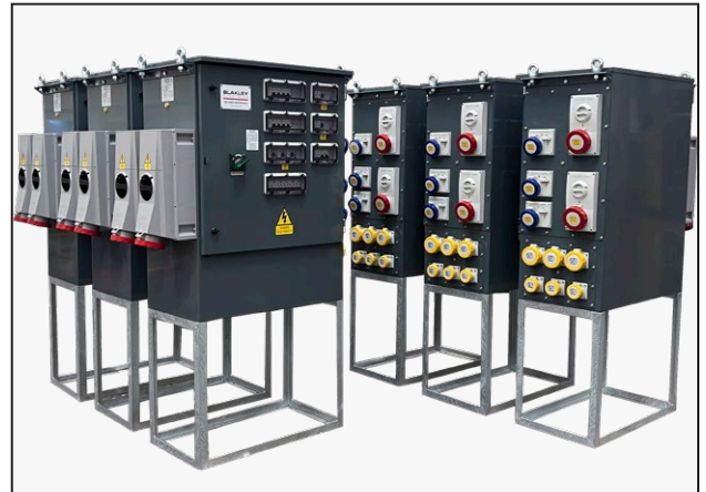
A7293318 General Purpose Multiplex Outlet Panel, 400A Fitted 125A & 63A 400V 5P Sockets, 16A & 32A 230V 3P Sockets and 16A & 32A 110V 3P sockets fed from an integral transformer
