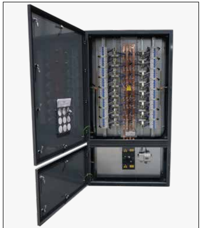
A7293373 Distribution Board with 250A 4P incoming switch and 16 no. 40A 4P / 30mA DC Immune MRCDs. Shield plates removed.
