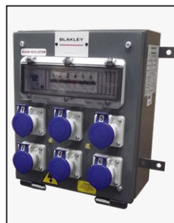
PC Assemblies, IP44, c/w 6 x 16A 230V (A7291176) & 1 x 32A 400V & 1 x 16A 230V (A7292234)
