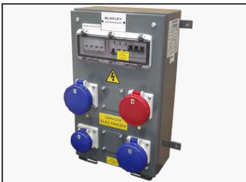
PC Assembly, IP55, c/w 1 x 32A 400V, 2 x 32A 230V and 1 x 16A 230V socket, Part No. A7291178
