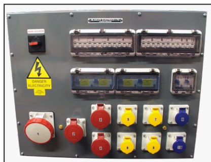
PC Assembly, IP44, c/w 1 x 63A & 3 x 32A 400V, 2 x 16A 230V & 4 x 16A 110V, Part No. A7291597
