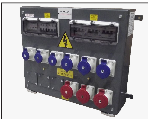
PC Assembly, IP44, c/w 3 x 32A 400V, 3 x 32A 230V and 3 x 16A 230V sockets, Part No. A7291179
