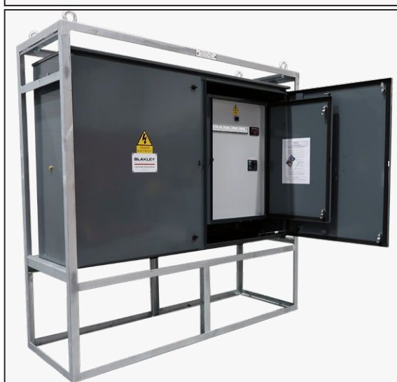
Part A7292369 Shore to Ship Assembly, providing 110V RLV and 400V LV supplies for vessels. Cables with plugs enter through the underside via brushed strips. Enclosure fabricated from 316L stainless.
