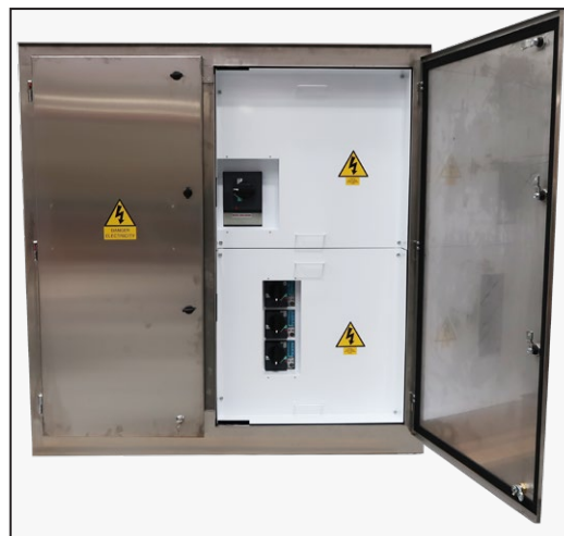
A7292330 MCCB Panelboard, Brushed Stainless Enclosure, 400A, 6 way with Ethernet Gateway
