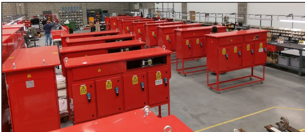
Final Assembly of 20 no. 400A Form 4 Type 3 Mains Distribution Assemblies nearing completion. Enclosures are fabricated from 316L stainless steel with a conspicuous painted finish, shade Poppy Red to BS4800 04 E 53.
