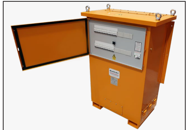
Part A7030972R - incorporating a 20kVA transformer, 17 no. outgoing DP MCBs protected by a DC immune RCD.
