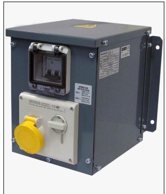
Switch on socket cannot be turned to the ON position until a plug is inserted and so there are no off-load losses.
