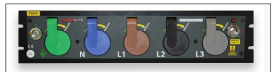
Optional sequential powerlocks where connectors must be connected / disconnected in sequence (earth is first in and last out)
