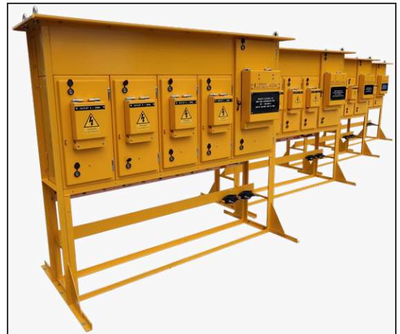
Part Number A7292936, Dockside Service Unit, rated at 800A with 4 no. outgoing feeders rated up to 400A
