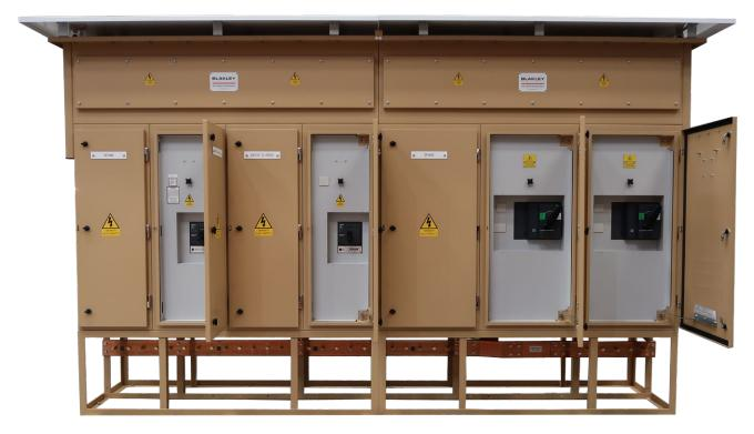
Part No. A7193465 incorporating 3 no. 800A 4P incomers, supplying distribution switchgear via 2200A bus bars. The assembly was provided with a separate stand extension, increasing the ground clearance to 1 metre.
