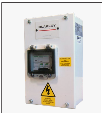
ELE Series Type A RCD Assemblies, Double Pole or 4 Pole, Fixed or Variable Sensitivity, up to 125A rating
