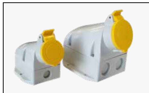
16A and 32A, 110V, 2P+E, IP44, Surface Sockets
