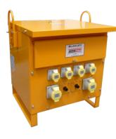
Rated at 10 kVA, incorporating sockets to feed power tools and hard wired connections to feed dedicated 3 core lighting circuits. Sockets are MCB protected and hard wired circuits are MCB or MCB / RCD protected. Transformers have a 110V RLV output.
