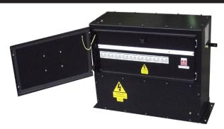
Combines a step-down, double-wound transformer with a double-pole MCB distribution arrangement and utilises a double-wound transformer with dual 55V secondary windings to LUL specification. The assembly provides a 110 volt Reduced Low Voltage Supply.
