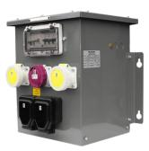
Single Point Distribution Assemblies are factory built assemblies supplied complete with different combinations of switchgear, transformers and socket outlets rated at 230V, 110V and 24V. The standard range of SP assemblies is available with ingress protection of IP20, IP44 or IP55
