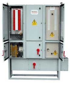
Assemblies typically comprise of 3 no. vertical sections, each incorporating a main isolator, a 110V step-down 6kVA transformer and a 12 way MCB board suitable for DP MCBs. An optional Master Isolator can also be incorporated.
